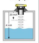
**E. Maximum Applied Range:** The Individual or cumulative effects of agitation, vapor or foam can reduce the overall quality of signal return and shorten the maximum applied range of the transmitter. To determine the maximum applied range of the transmitter in your application, refer to the below derating chart.
